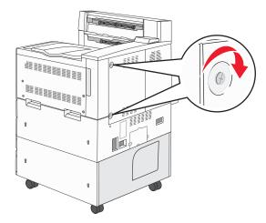
4 Plug the printer power cord back into a properly grounded electrical outlet and turn on the printer.
